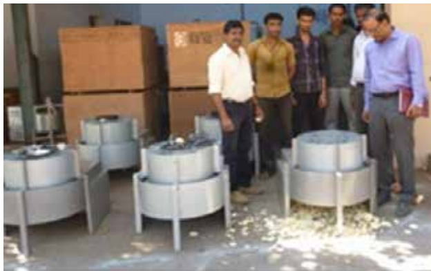
Fig. 76. Motorised cassava chipping machine
