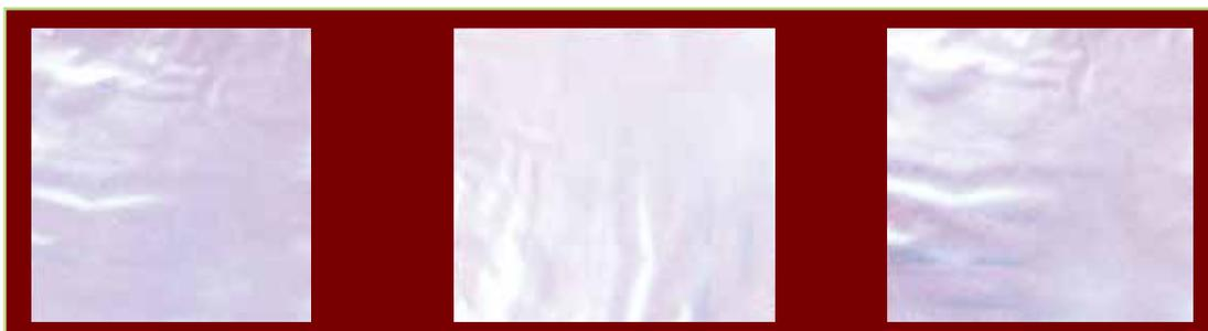
Fig. 80. Biodegradable films from modified starch-wax composites
