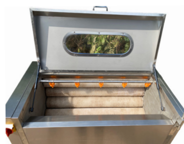
Fig. 51. Multipurpose peeler for taro and sweet potato
