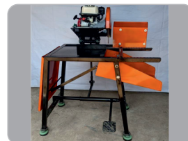
Portable self –propelled cassava sett cutter
