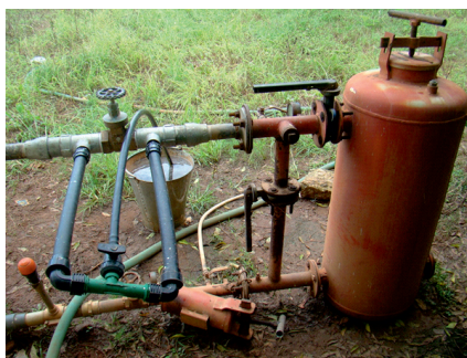
Photo 14. Venturi based drip fertigation system
