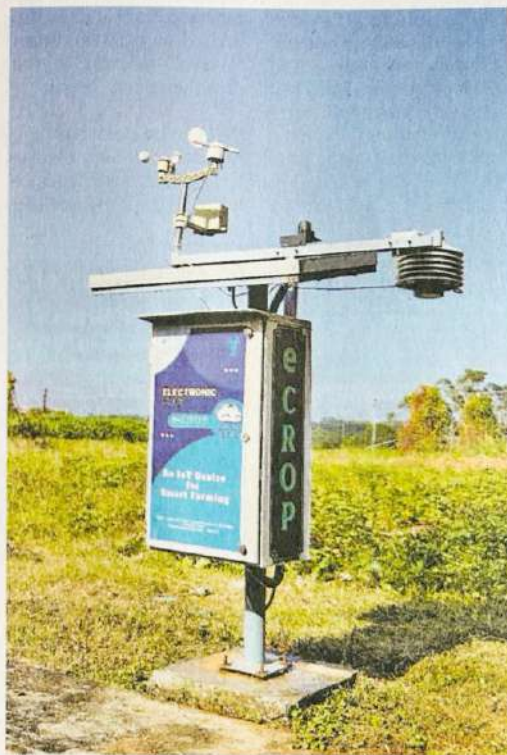
The e-Crop device developed by the ICAR-Central Tuber Crops Research Institute.
